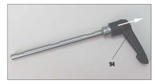
instrument and knife holders can be turned to the position that is most convenient for each user. Pull the grip (94) out of the lever, hold it in this
